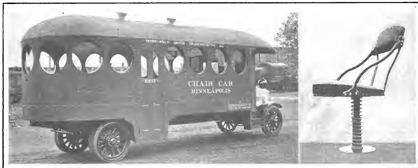
Left—McKeen-United Highway Coach. A luxurious chair car on a 3½-ton chassis, intended for interurban transportation. Right—Chair used in Highway Coach. Observe the very long coil spring which supports the weight
